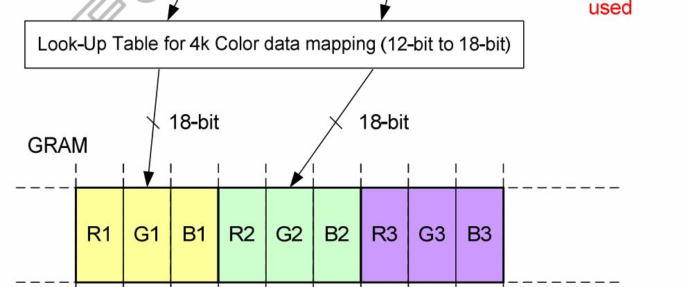
The diagram illustrates the data flow for writing RGB 4-4-4-bit data into GRAM. The input bits D7-D0 are mapped through a LUT to produce 18-bit values, which are then written into the GRAM. The GRAM is represented as a 10-bit wide memory with columns labeled R1, G1, B1, R2, G2, B2, R3, G3, B3. A red arrow points from the LUT output to the GRAM, with the text "R23~R20 will be late and are not used".
