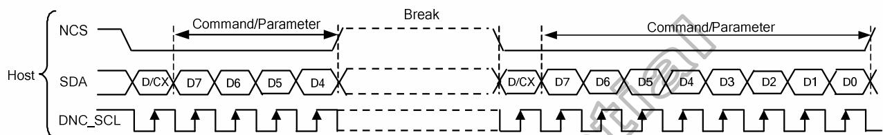
**Figure 5. 31 Display Module Data Transfer Recovery**
