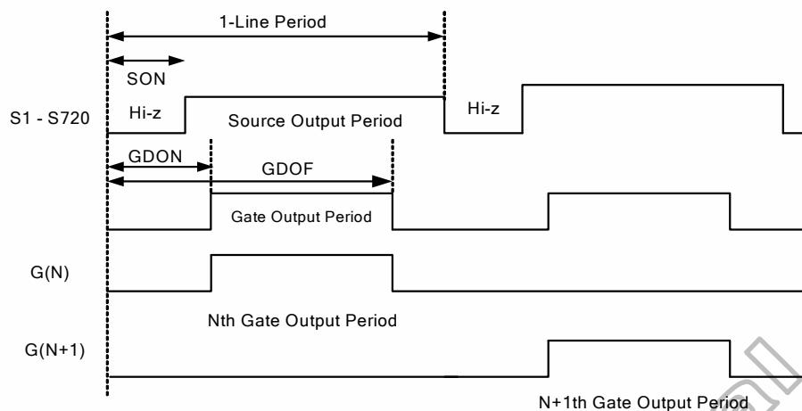
**SON7-0:** Specify the valid source output start time in 1-line driving period. The period time is defined as SYSCLK clock number. (Please note that the setting "00h" and "01h" is inhibited).
