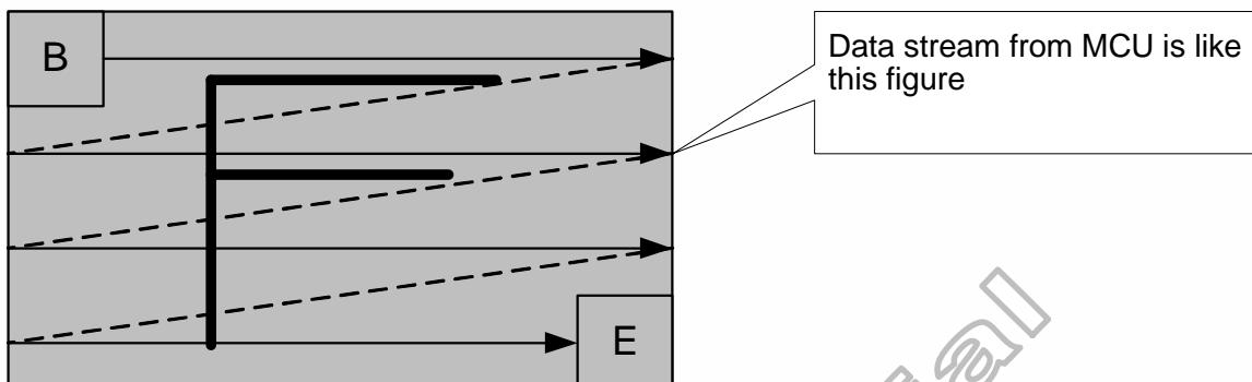
Figure 5. 32 MCU to memory write/read direction
