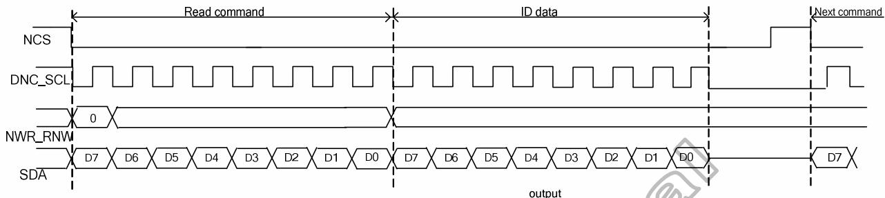
24 bit Reading function with including dummy clock
