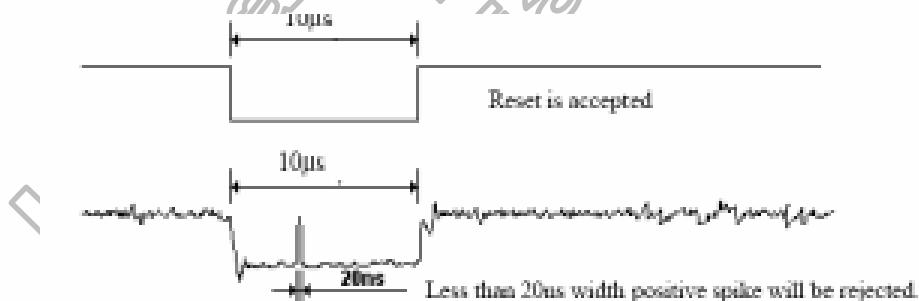
(5) It is necessary to wait 5msec after releasing NRESET before sending commands. Also Sleep Out command cannot be sent for 120msec.
