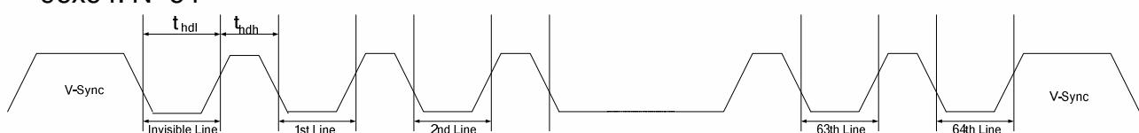
**Figure 5. 46** $t_{hdh}$ = The LCD display is not updated from the Frame Memory $t_{hdl}$ = The LCD display is updated from the Frame Memory (except Invisible Line – see above.)
