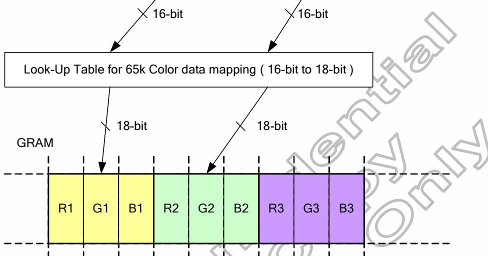
Figure 5. 19 Write data for RGB 5-6-5(65k colours) bits input in 9-bit parallel Interface (when support Look-up table and LUT\_EN=0)
