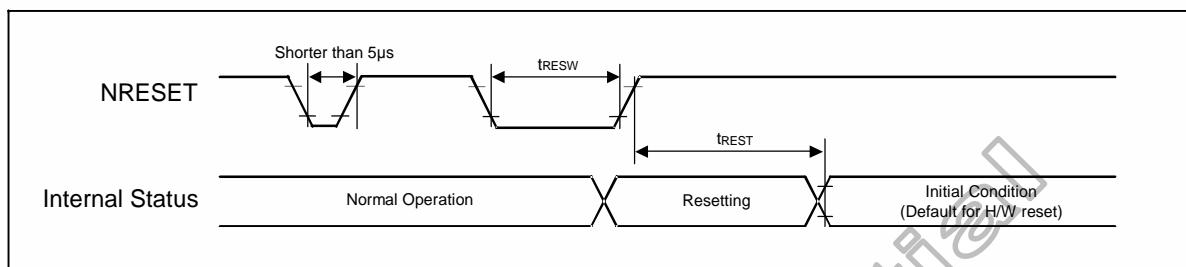
**Figure 7.5 Reset input timing**
