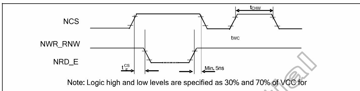
**Figure 7. 2 Chip select timing**
