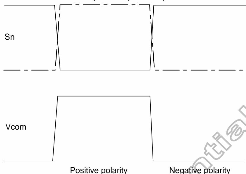
**Figure 5. 58 Relationship between Source Output and Vcom**
