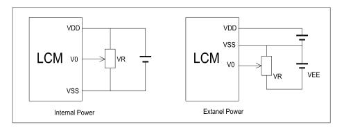
$V_{DD-V_0}$ : LCD Driving voltage VR: 10k~20k
