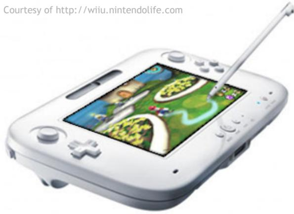
The resistive touch panel is made up of several layers. When you press down onto the touch panel with your finger or stylus, the top layer flexes and pushes back onto a layer behind it. This will effectively complete a circuit and tell the controller which part of the touch panel is being pressed.
