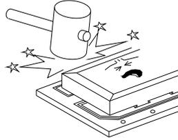
LCD may be shifted or conductive rubber may be reshaped, which will cause defects.
