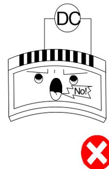
**Do Not Put Pressure on the Metallic Frame or Disassemble the LCD Module**
